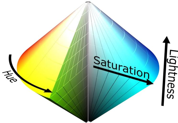
There are 3 dimensions that can be adjusted, Hue, Saturation and Lightness. To simplify the operation, Saturation can be set to a fixed value.
