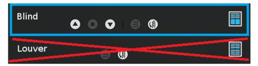
Unfortunately the Navigators don't hide the Louvers field if the connection is done, that has to be done via the room properties in Composer (hide the louver part of the blind) To get the 2 fields merged, simply connect (in Connections) the binding BLIND\_SECONDARY\_CONTROL and refresh Navigators
