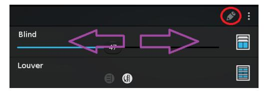
Be aware that the blind have feedback from the slider position and will show an unknown position each time the Controller starts up. As well the toggle buttons will show a question mark. In this status the driver is *uncalibrated*
